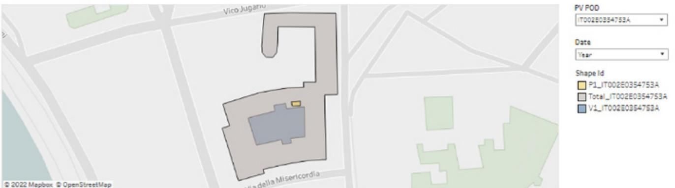
Map shows Via Luigi Petroselli building in municipality #1. It has a total rooftop area of 3,667 m2. Currently, 16 panels are installed in 17.00 m2 area of the rooftop. The total capacity of the plant is 1.920 kWp. This building has 350.1 kWp of unused PV potential.
