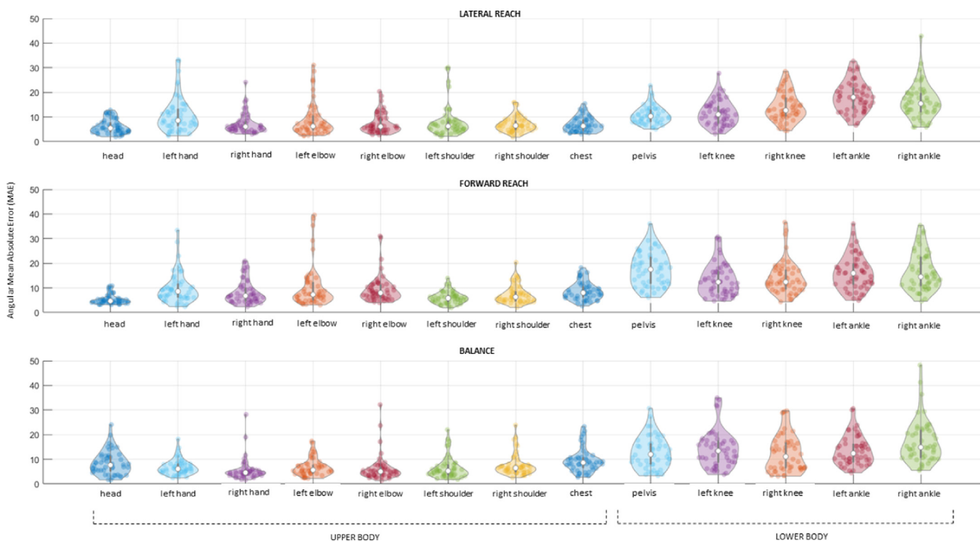
Fig. 12. Violin plot of the angular Mean Absolute Error (MAE) for the body tracking analysis. The upper subplot refers to the joints tracked during the lateral reach exercise, the middle subplot to the forward reach test, while the lower subplot summarizes the data for the balancing exercise.
