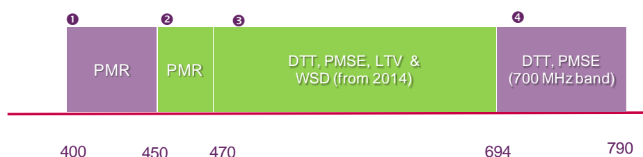
Figure 4: Illustration of spectrum use 400 – 790 MHz
