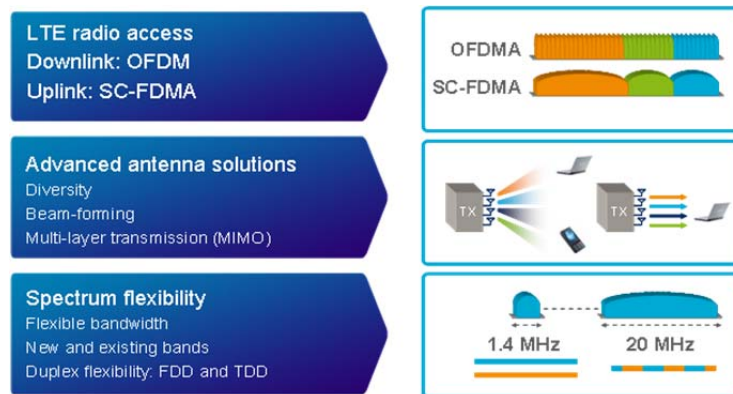
Figure 6-3: Key LTE Radio Access Features
