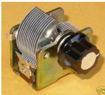
Figure 3-1: Traditional TV tuner with variable capacitor as used from 1940s to 1980s.
