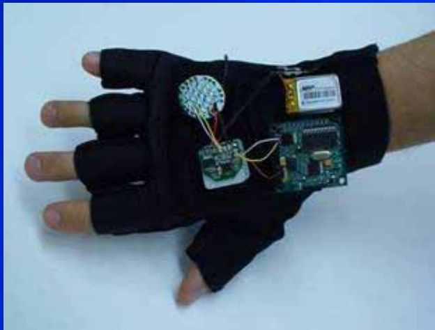
Integrated Reader & Mote-based iGlove (Intel Research Seattle Lab)
