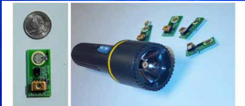
Fig. 1 Tag (with DIP-8 PIC12C509 shown here) and flashlight transmitter-interrogator
