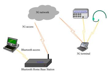
cases it may even be possible to leave the PC at home connected to the Home Base Station (via Bluetooth), and retrieve data from it directly to the bpad using Bluetooth and 3G together.
