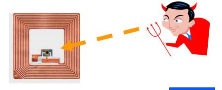
Attacker can derive the secret from the tag and make a clone • E.g. EPC Tag is easily cloned (Basically a Barcode) Research
